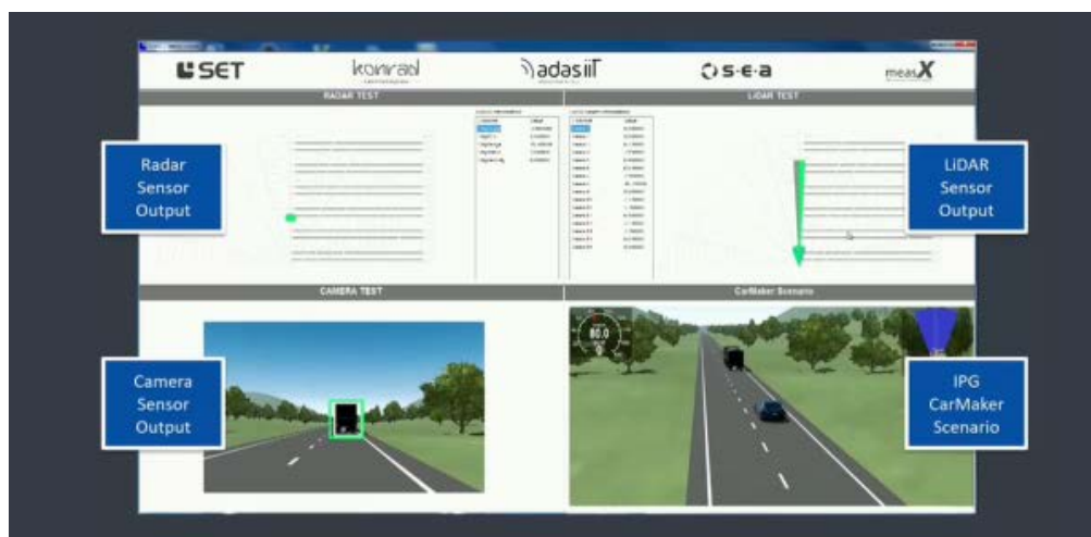
Figure 4: (From Bottom-Left, Clockwise): Camera sensor output, Radar sensor output, Lidar sensor output, and Scene generator simulator, IPG CarMaker all running in a closed loop for Sensor Fusion HIL test.
