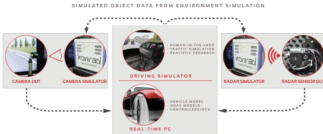
Figure 2: DIL with Sensor Fusion Test Top Level Architecture
