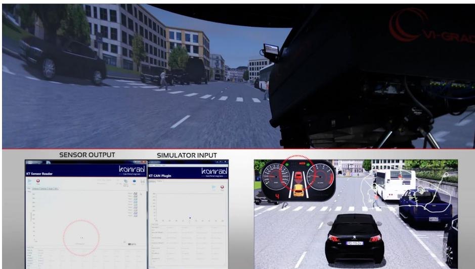
Figure 4: Automated Emergency Braking (AEB) Test with DiM150 and Sensor Fusion Test. Notice the positive correlation between the red circles showing the objects detected by the radar sensor and the red car indicator on the UI cluster.
