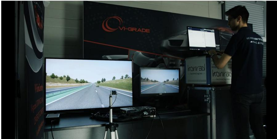
Figure 3: shows the radar and camera simulators connected to the DiM150.
