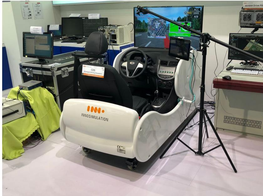
Figure 2: Compact Driving Simulator (CDS) from Innosimulation with the nVidia PX2 on its right and the Konrad Radar Object Simulator with GNSS and V2X simulators on the left.
